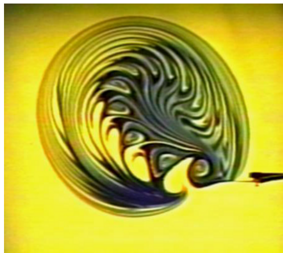
Fig. 2. Formed self-propagating coherent eddy at t = 60 s. The width of the frame is 30 cm.
